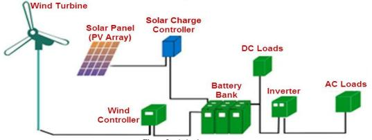
Figure.3: wind-solar system
