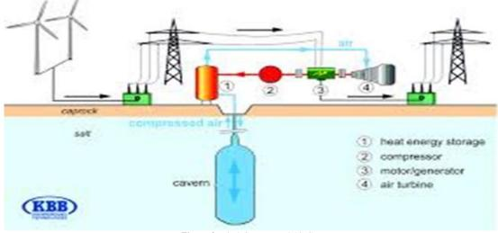
Figure.2 Wind-Compressed Air System
