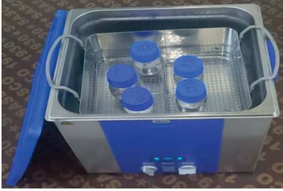
FIGURE 3. Suspension of \text{Al}_2\text{O}_3 in paraffin wax by ultrasonic water bath (Elmasonic P180H)
