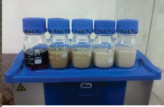
FIGURE 4. View of the pure paraffin wax and \text{Al}_2\text{O}_3 nanoparticle suspended in paraffin wax with concentration (0.5, 1, 3, 5) wt. %
